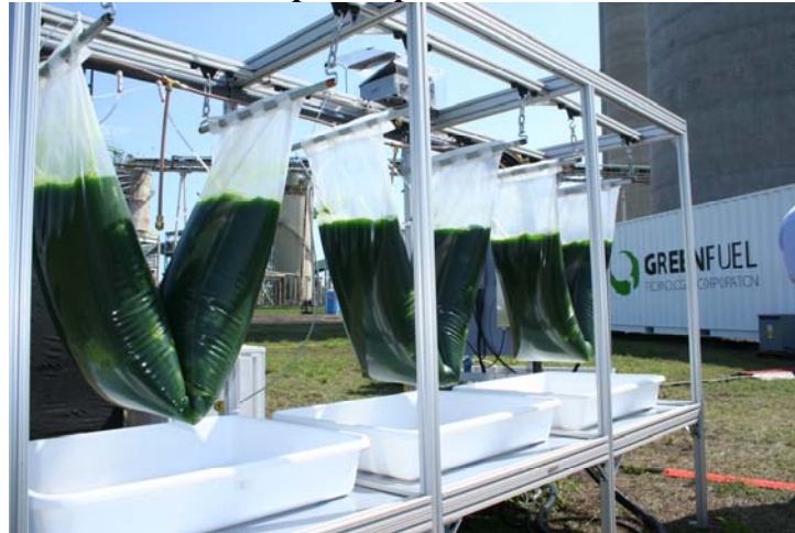
Figure 5. Operating demonstration algae bioreactor at a coal-fired power plant in Louisiana.
